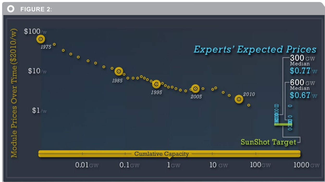
FIGURE 2: Falling prices for solar modules. As the total amount of solar modules produced has increased over the past few decades (from left to right), the price per watt has also fallen. Prices 1975-2009 are from Nemet (2009), and prices for 2010 and 2011 are based on data from Navigant and Bloomberg New Energy Finance. 5 Blue circles indicate the expectations from Near Zero’s survey, for solar module prices at 300 GW and 600 GW of total installations (also called cumulative capacity). Also shown for reference in green is the module price target of the Department of Energy’s SunShot Program.
